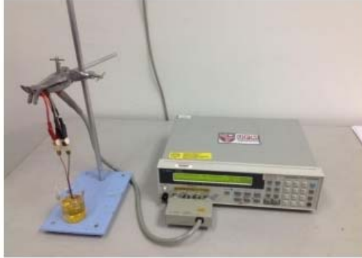
Figure 3: IDE impedance sensor probe connected to a LCR meter for impedance measurement.
