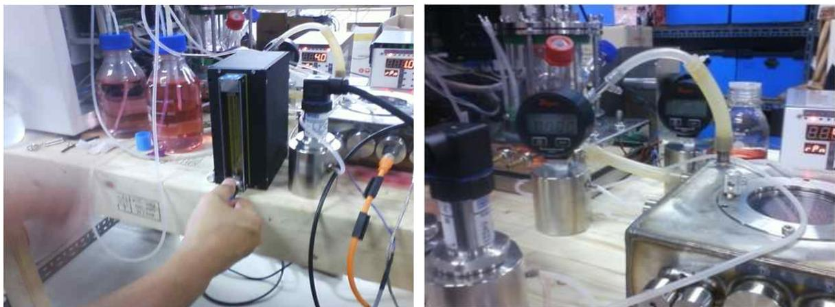
Fig. 8-12. Pictures of pressure controller for controlling internal pressure of culture chamber
