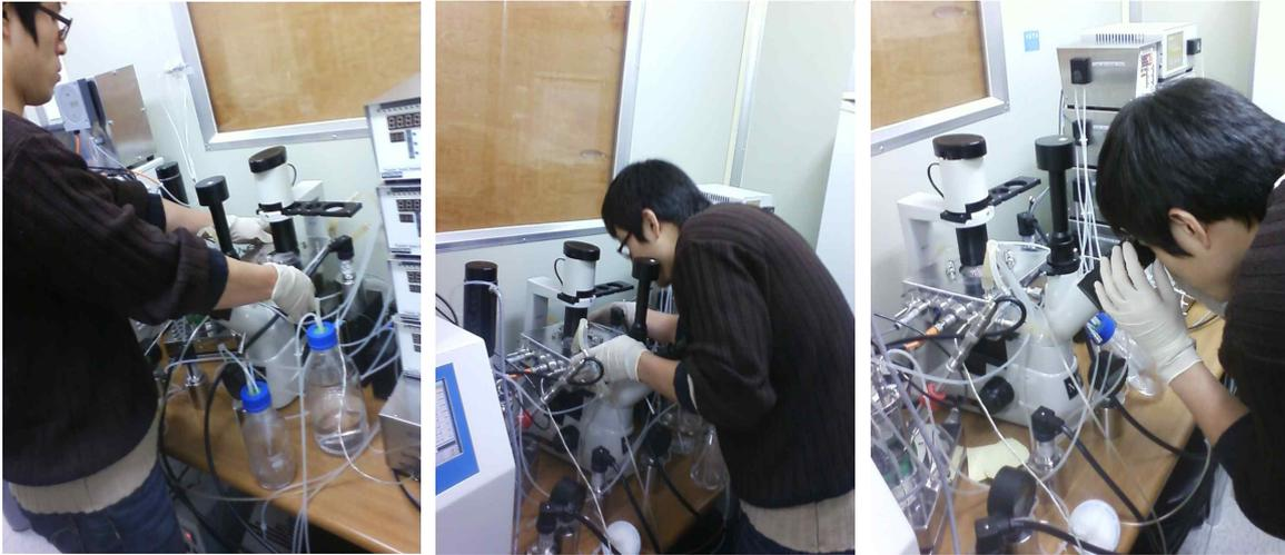
Fig. 8-18. Pictures of pressure controller for controlling internal pressure of culture chamber
