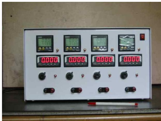
Fig. 4-1 Micro-electric supply composed of potentiometer, controlled timer, and monitor manufactured for this study.
