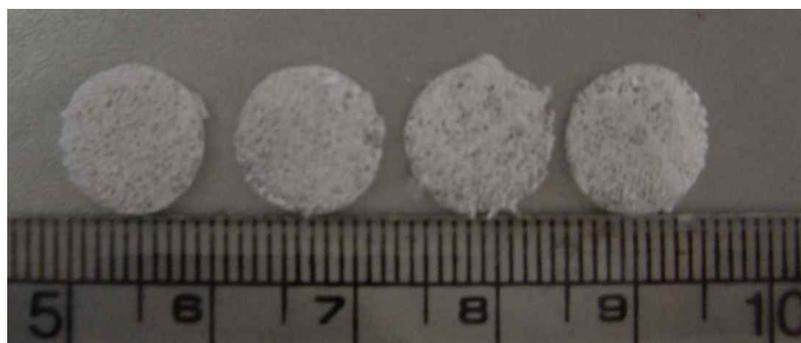
Fig. 2-5 A macroscopic image of composite bioceramic scaffolds prepared with gnotobiotic pig bone powder and P(D,L)LA using a solvent casting and NaCl leaching method
