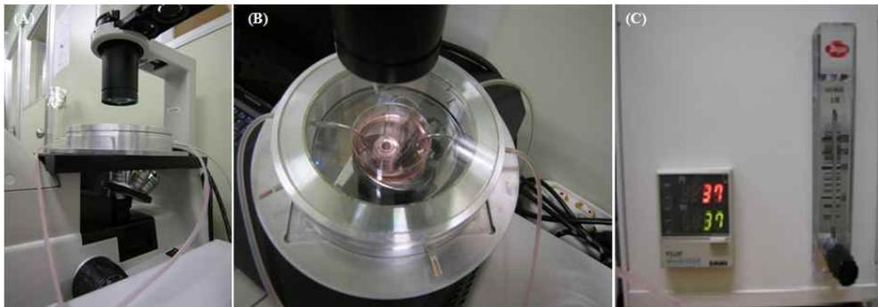
Fig. 7-3. A novel perfusion flow chamber system and its controller; (a) image of a novel perfusion chamber system on the microscope stage, (b) image of medium perfusion in a novel perfusion chamber system, and (c) temperature(37°C) and 5% CO<sub>2</sub> controller
