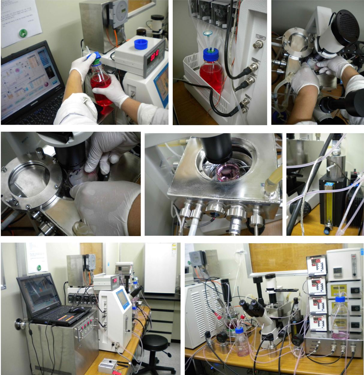
Fig. 8-17. Pictures of cell culture process via the developed perfusion culture system
