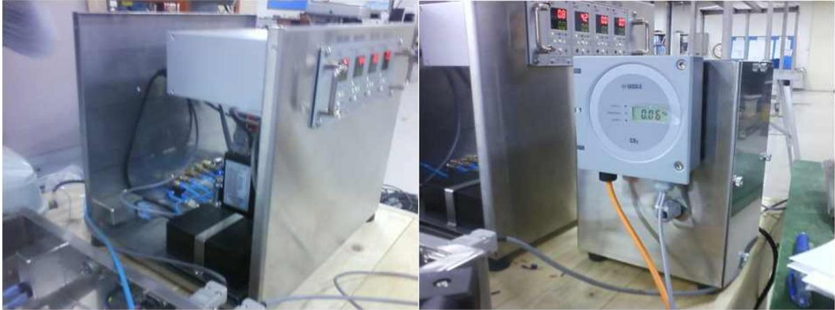
Fig. 8-6 Validation of a 4 gas mass flow controller(air, N<sub>2</sub>, CO<sub>2</sub>, O<sub>2</sub>) of a perfusion flow culture system made at the BIOTRON Inc.
