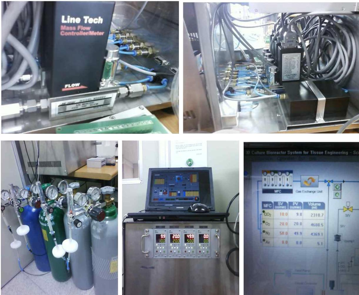
Fig. 8-11 Pictures of 4 gases mass flow controller (air, N<sub>2</sub>, CO<sub>2</sub>, O<sub>2</sub>)
