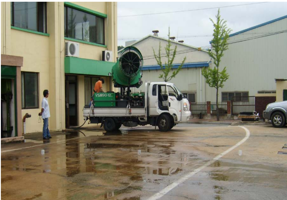
<Fig. 4-30> A feature of preparation of testing spray quantity
