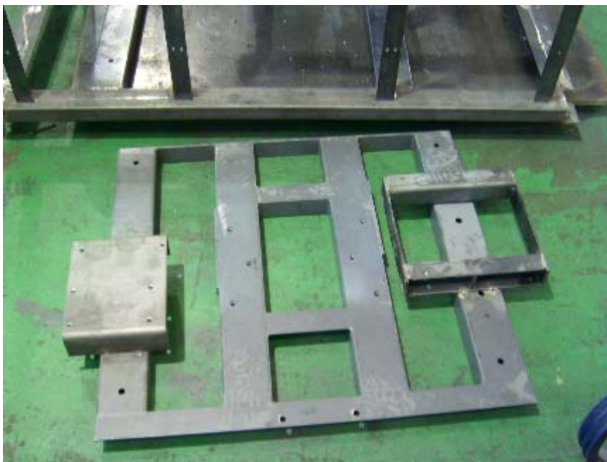
<Fig. 3-25> Water meter and spray pump fixing frame
