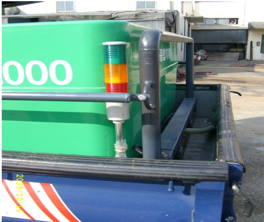
<Fig. 3-57> Signal processing equipment for adjusting quantity of pumping water
