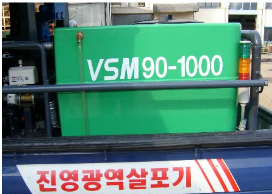
<Fig. 3-28> Install on water tank vehicle
