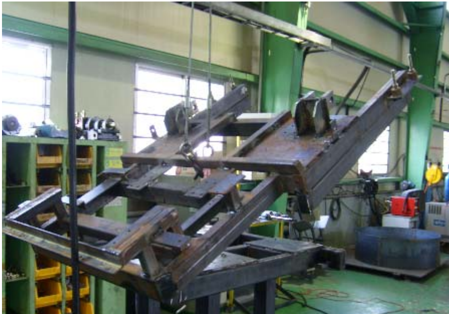
<Fig. 3-23> Adjustment device of the height of up and bottom of a wind blowing fan
