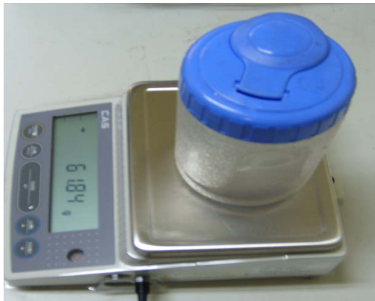
<Fig. 4-47> Measurement of spray quantity
