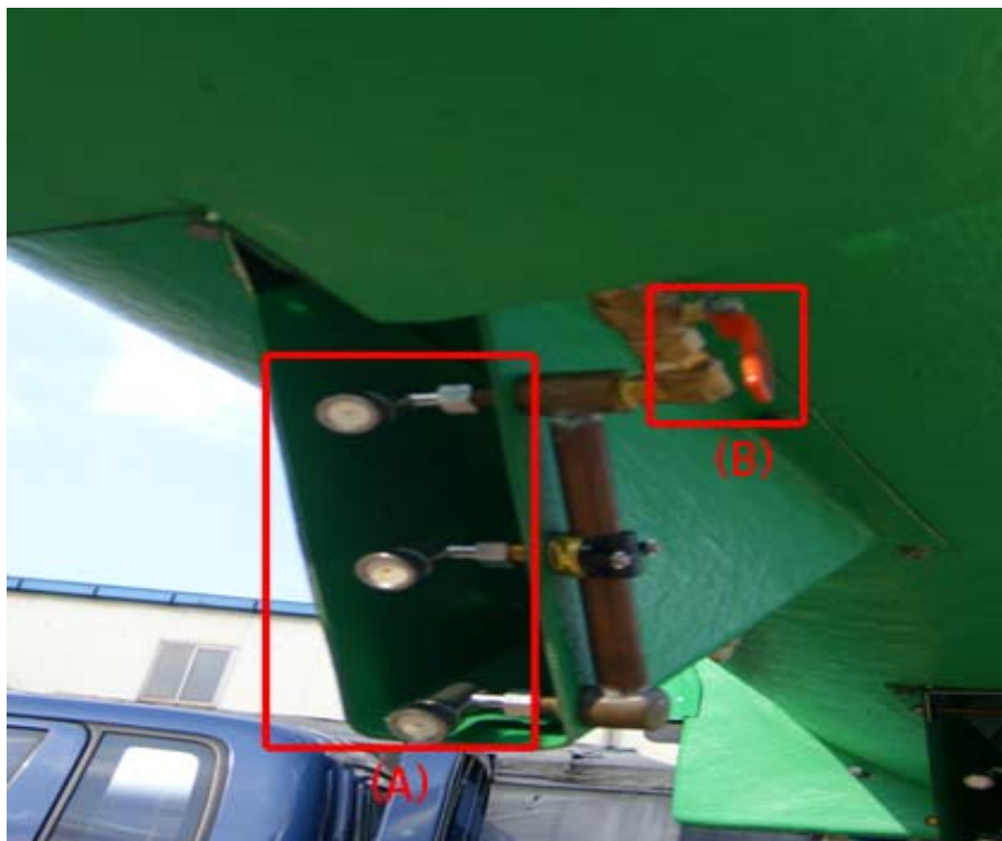
<Fig. 3-44> Three nozzles in lower part
