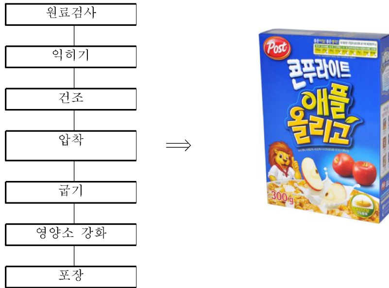
Fig. 5-16. Production process of "cereal" using "RP 70".
