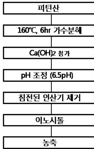
Fig. 2-3. Production process of inositol extraction from phytic acid.
