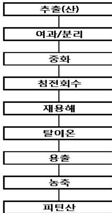
Fig. 4-7. Production process of phytic acid isolation from Defatted rice bran.
