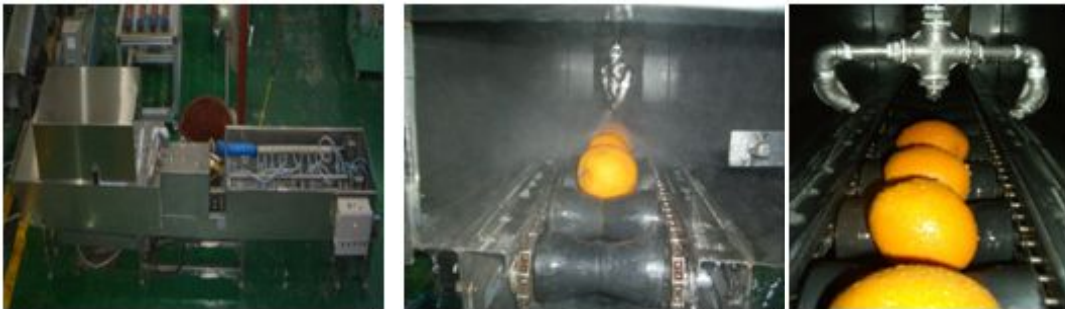
Fig. 4. Mechanical washer system.
