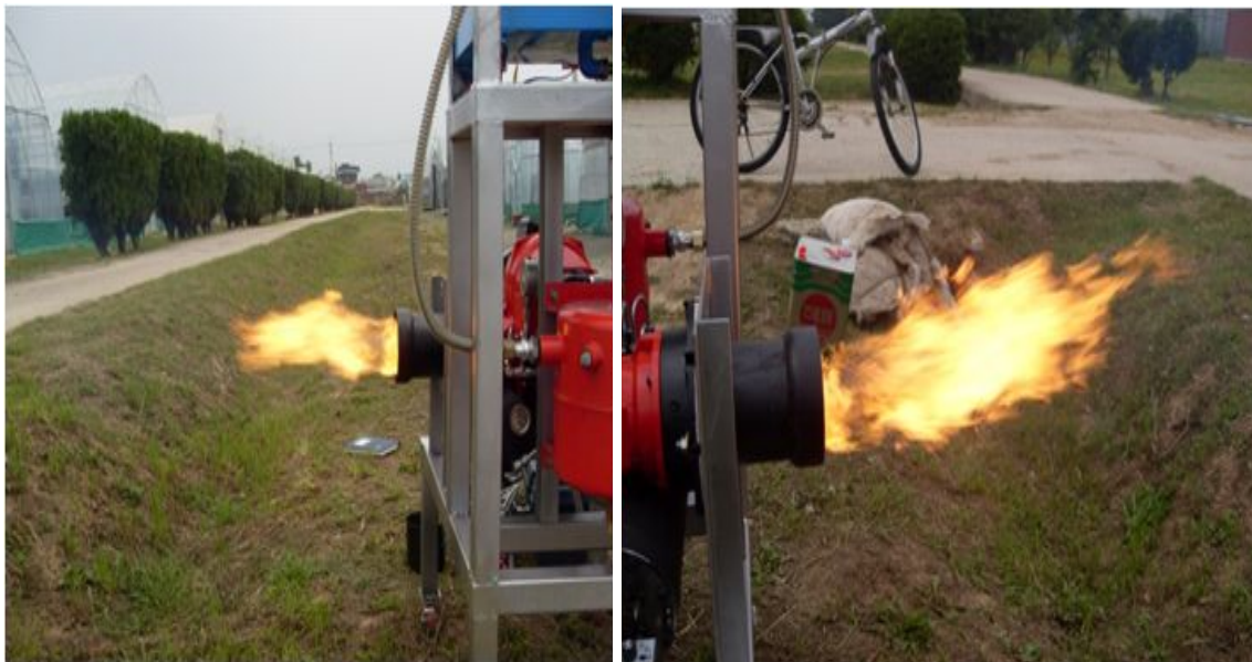
Fig. 13. Fuel spraying burning test
