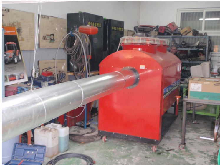
Fig. 19. Picture of hot air heater using waste edible oil
