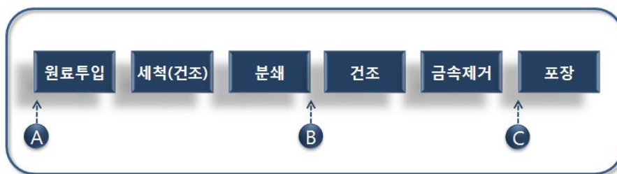
Fig. 22. Data collection for microbial contamination during red pepper powder processing for probabilistic risk modeling.
