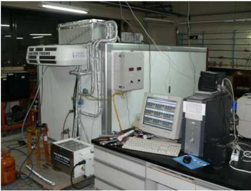
Photo 3 Refrigeration system using sliced raw fish transportation.
