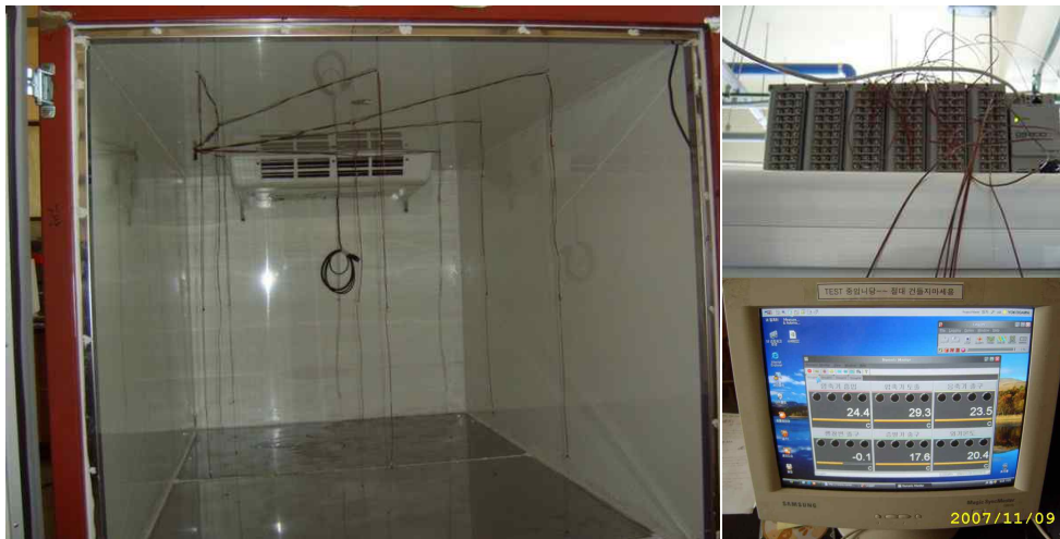
Photo 2 Attachment of temperature sensors in experimental apparatus for refrigerated vehicle development.
