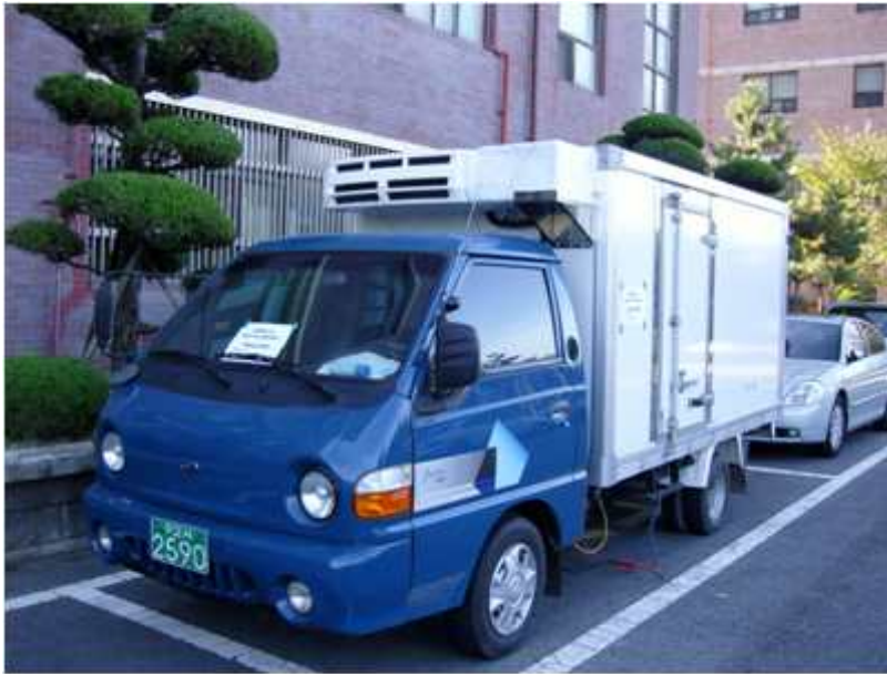
Photo 4 Refrigerated vehicle with heat storage installed.
