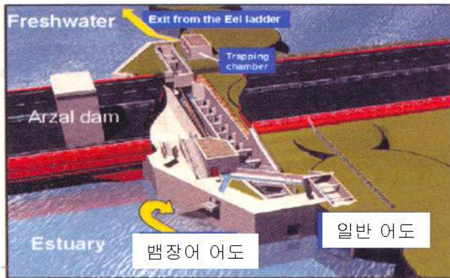
Fig. 7. Fish ladders in Vilaine River estuary in France (from Fontenelle et al. 2001)
