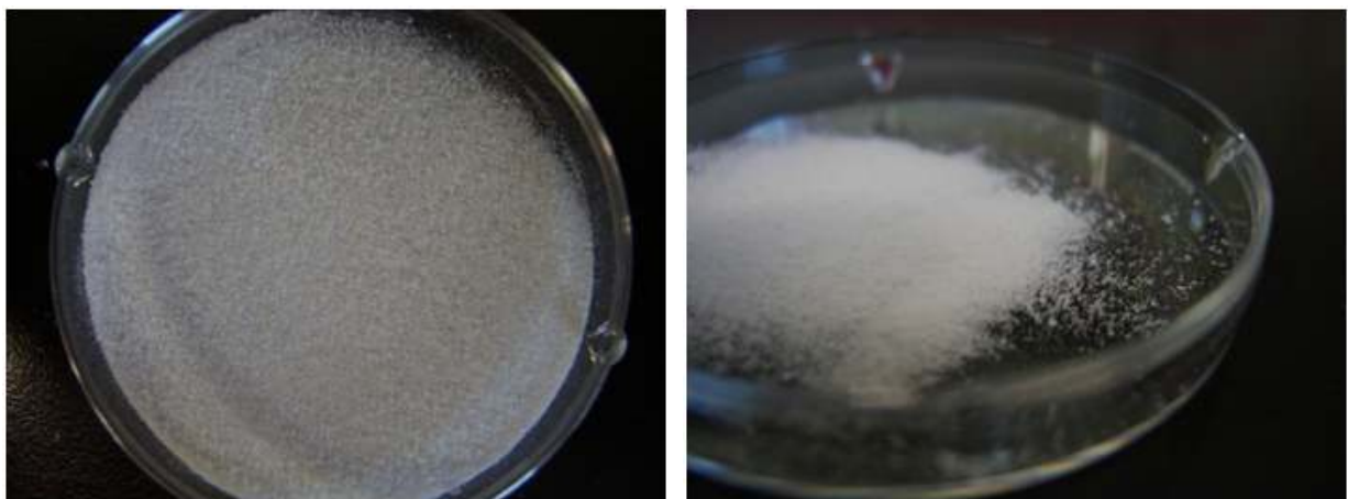
Fig. 8. Photographic representation of microcapsule powder containing perilla oil under the conditions optimized in this study.
