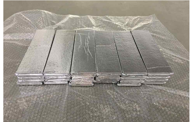
알루미늄증착2중지/알루미늄증착2중지 /fumed silica (front/back)
