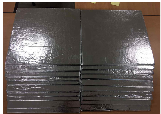
HD95/HD95/board type fumed silica
