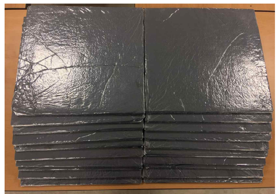
HD95/HD95/board type fumed silica
