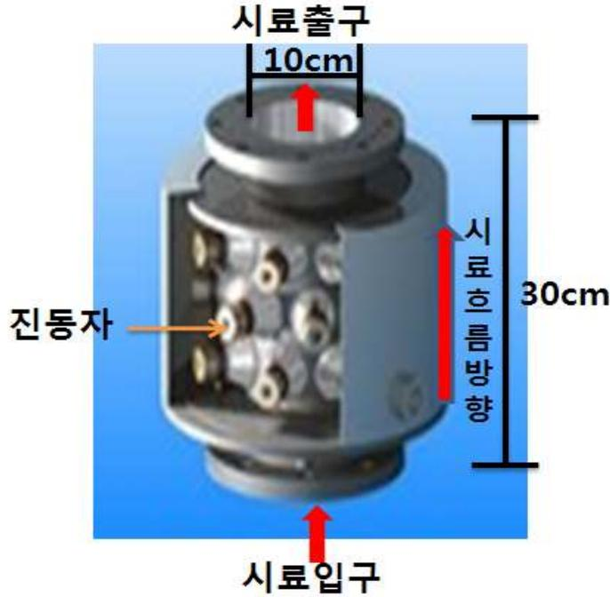
Fig. 54. Inner structure of ultrasonic wave generator
