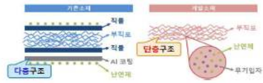
Fig. 3 Cross section of Multi layer screen & Non-woven screen
