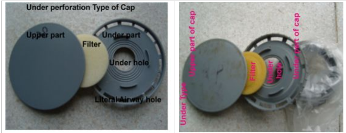
Fig. 0. Upper-Under and Under perforation cap type of polypropylene bottle & Upper-Under and Under perforation cap type of polypropylene bag.
