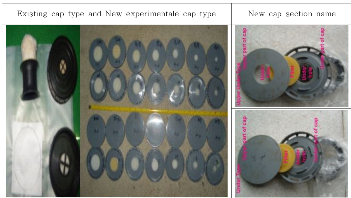
Fig. 1. Existing cap type and New experimental cap type & Upper-Under and Under perforation hole type of cap.
