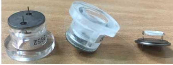
25MHz QCM chamber substrate
