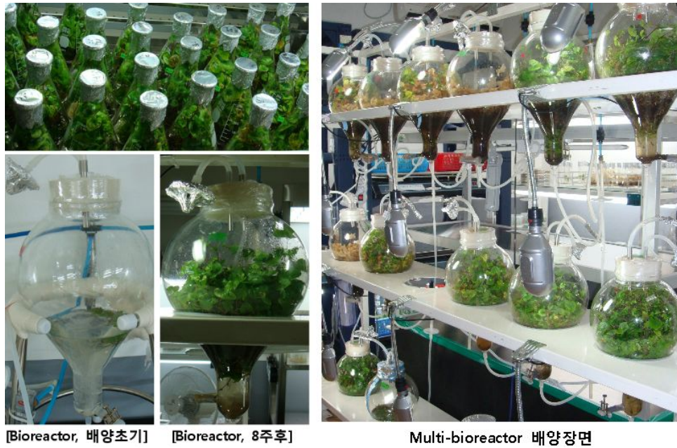
Fig. 8. Bioreactor culture of yam shoots using single node culture method.
