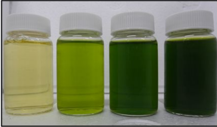
그림 77. Image of supernatant after centrifuging treatment from nanosuspension of chlorella (Dilution : 10 times, Pressure : 80 MPa)
