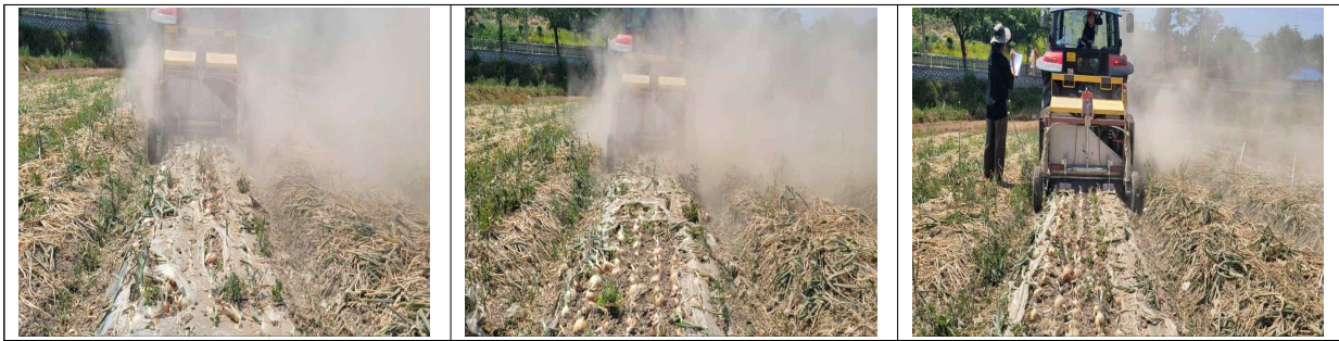
(a) PTO 1000(엔진 RPM 1600) (b) PTO 1000(엔진 RPM 1800) (c) PTO 1000(엔진 RPM 2000)
