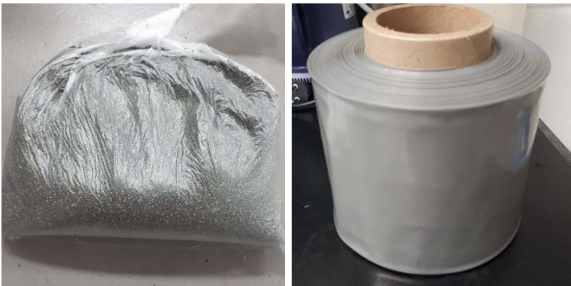
그림. 43. LDPE/Mel/ZnONP/GSE master batch and nanocomposite film.
