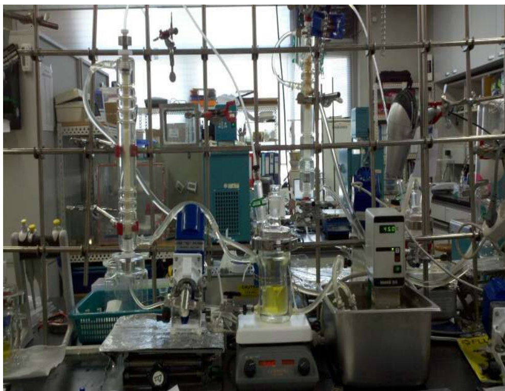
Figure 2. Lab-scale recycling PBR system for ethanolysis reaction.
