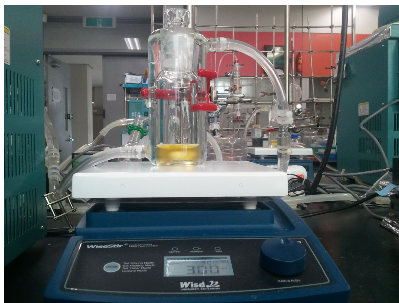
Figure 8. Reaction system for production of monoglyceride by enzymatic esterification.
