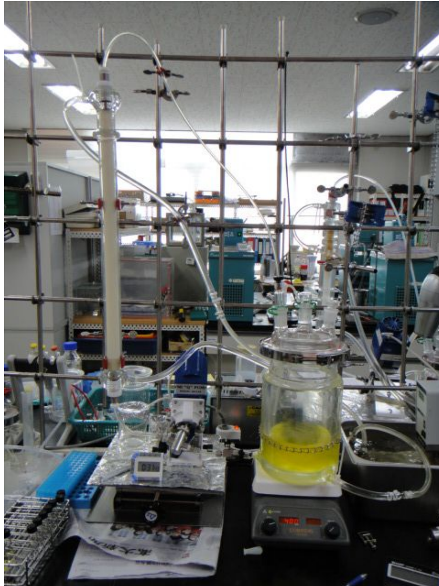
Figure 3. Bulk-scale recycling PBR system for ethanolsis reaction.
