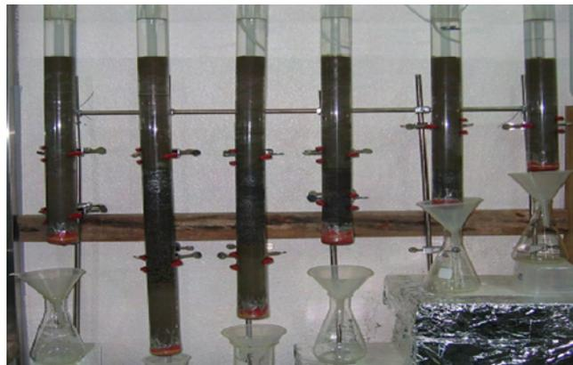
Fig. 32 Multi-layered soil columns used for measurement of hydraulic conductivity
