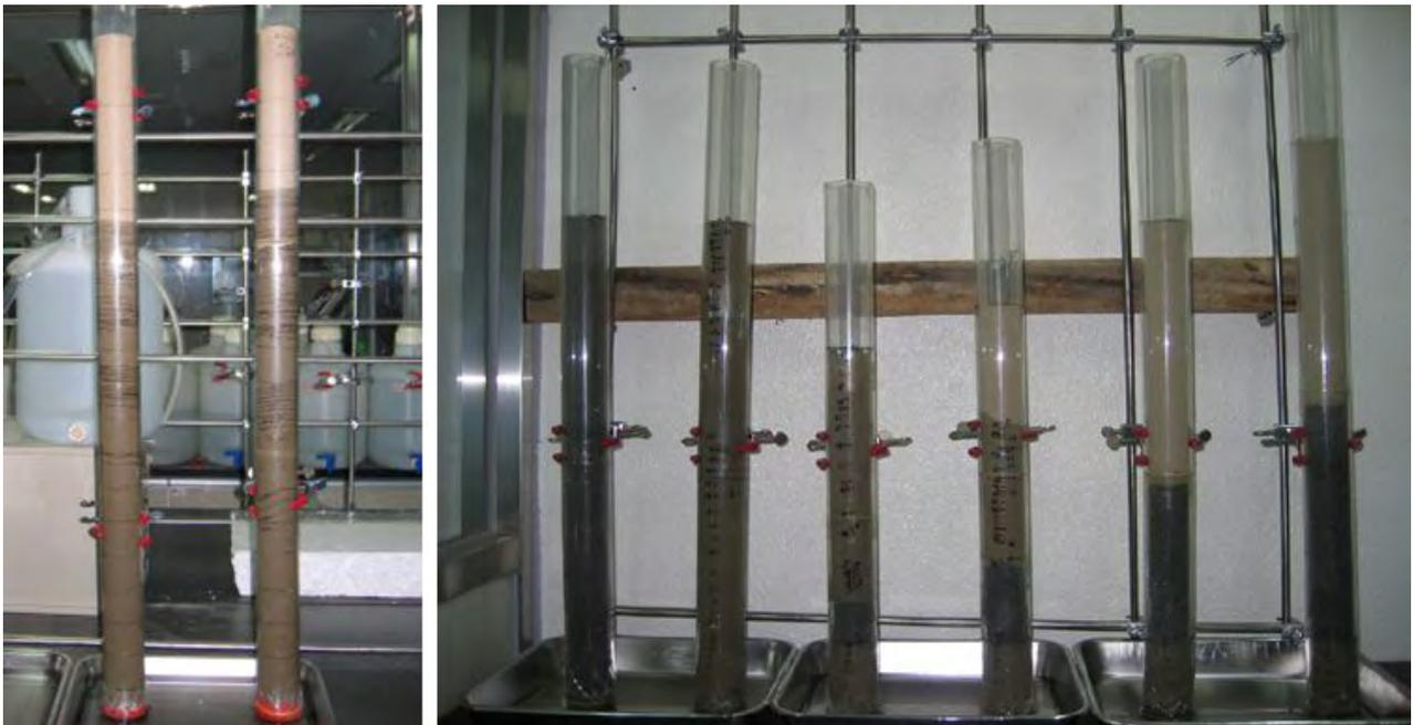
Fig. 33. Soil columns used for capillary rise experiment for mono- and multi-layered soils.
