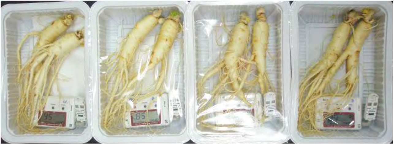
Fig. 3-35. Treatment for prevention of moisture condensation in tray with absorbents Non-woven fabric, 1/2 Non-woven fabric, Silicagel, Control
