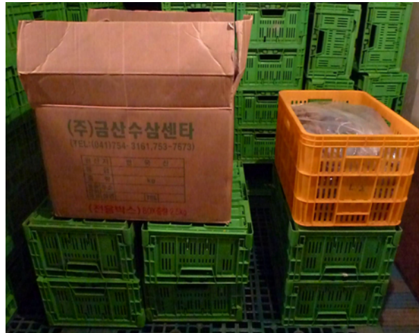
Fig. 2-27. Treatments for temperature measuring in ginseng boxes during precooling (Corrugated box: 75kg, Plastic box: 15kg)
