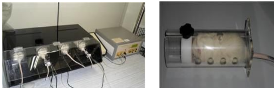
Fig 18. LE5002 storage pressure meter and a fake rat tail with cuff, sensor and restrainer
