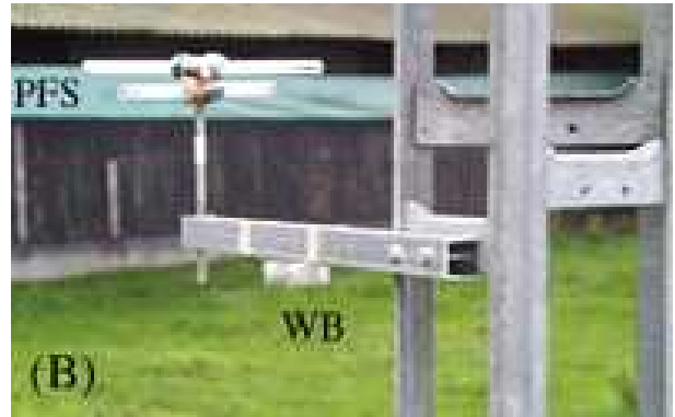
(b) Passive sampling techniques; WB = passive diffusion sampler; PFS = passive flux samplers
