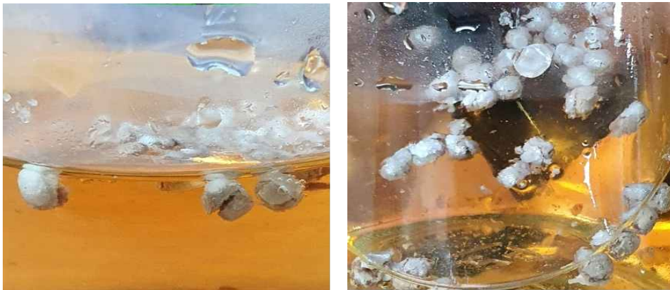
Fig. 21. The amino acids coated by lauric acid after 24 hours incubation on PB buffer (Experiment 1)
