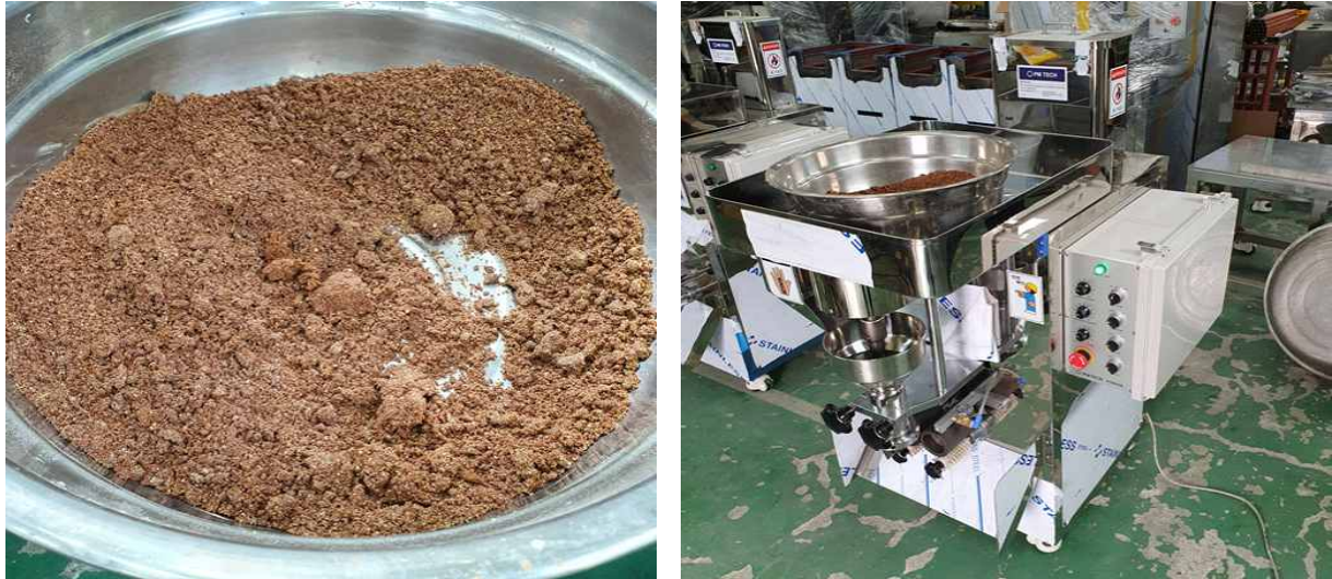
Fig. 16. Manufacturing process of rumen-protected nonessential amino acid
