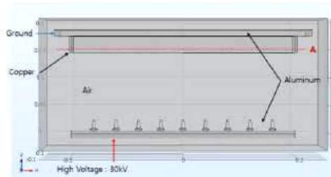
Fig. 2 Condition for electric field analysis
