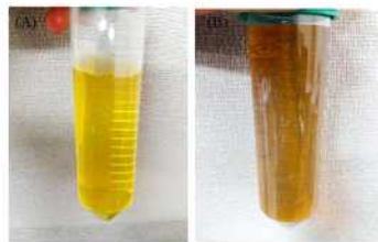
Figure 1. Photographs of the nanoparticles at different times. (A) Light yellow solution when 2mL of silver nitrate is added to 30mL of sodium borohydride solution. (B) Bright yellow solution when 10mL of silver nitrate solution is added to 30mL of sodium borohydride solution.
