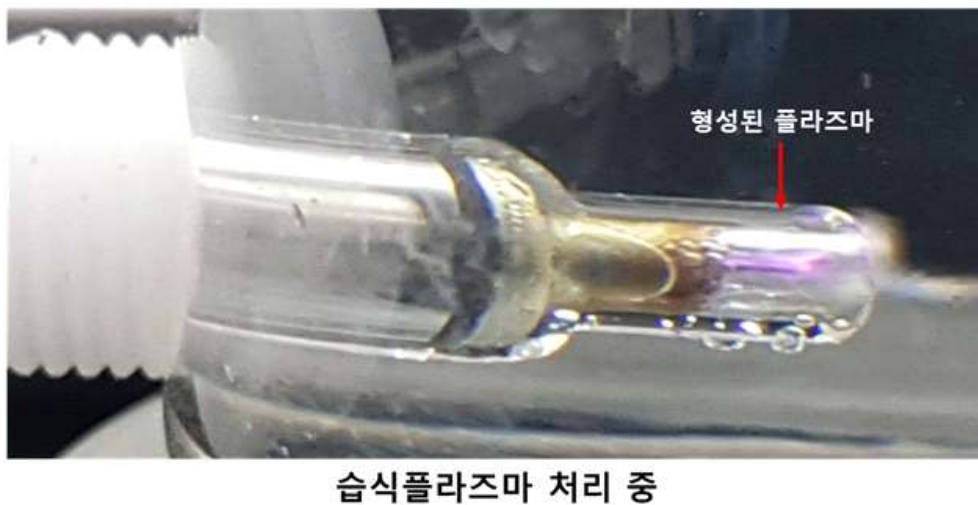
Fig. 5-2. Actual appearance of underwater plasma treatment.
