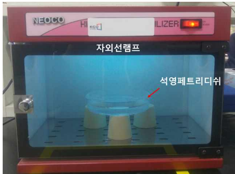
Fig. 5-3. Equipment of dry UV-C irradiation treatment.
