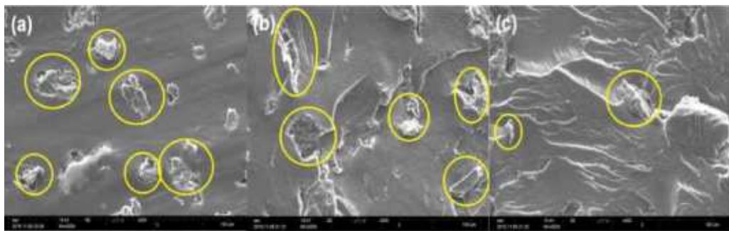
[그림] SEM images of: (a) LDPE/MCC composite; (b) LDPE/MCC-APS composite; (c) LDPE/MCC-TPPI composite.
