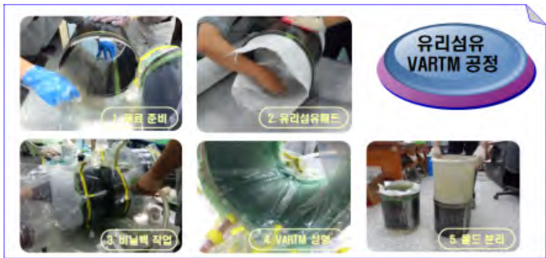
Fig. 60 Manufacturing process of GFRP
