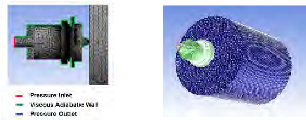
Fig. 86 Numerical grid for in/out side of Arc nozzle and boundary conditions
