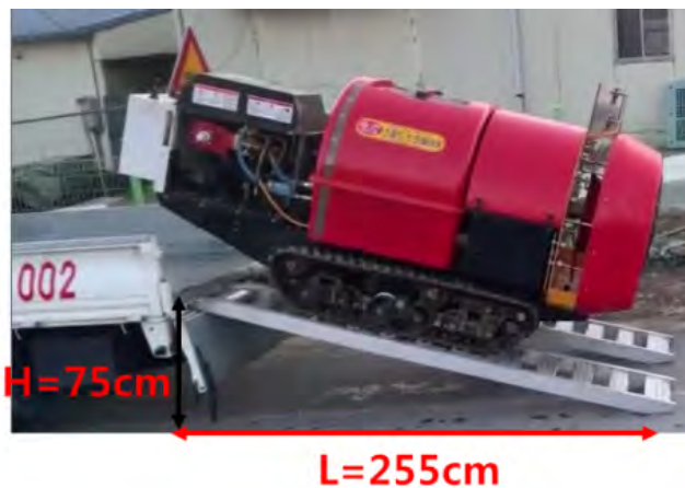
Fig. 103 The measurement on the gradeability of the speed sprayer
