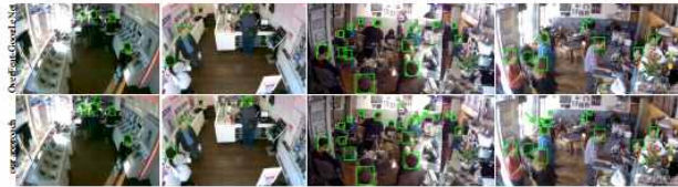
Figure 6: Example detection results obtained with OverFeat-GoogLeNet (top row) and our approach (bottom row). We show each model's output at 90% precision. See the text for a description and the supplemental material for a video 2 of our model's output.
