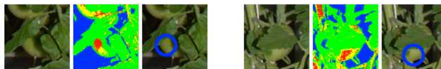
Figure 11. Examples of fruit detection under difficult conditions. The original images are to the left. The middle images show the results of pixel-based segmentation. The images to the right show the results of fruit detection.
