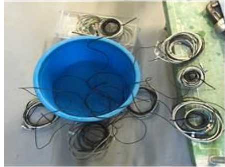
(b) Saturating pore pressure transducers
