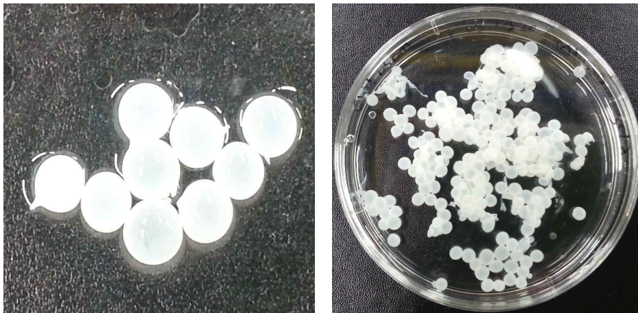
Figure 49. Chitosan bead formation
