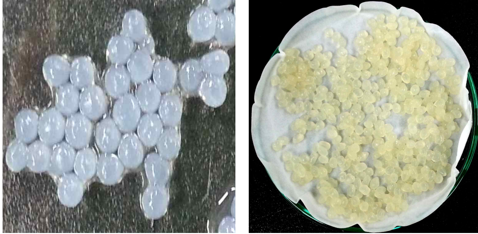
Figure 50. Alginate bead formation
