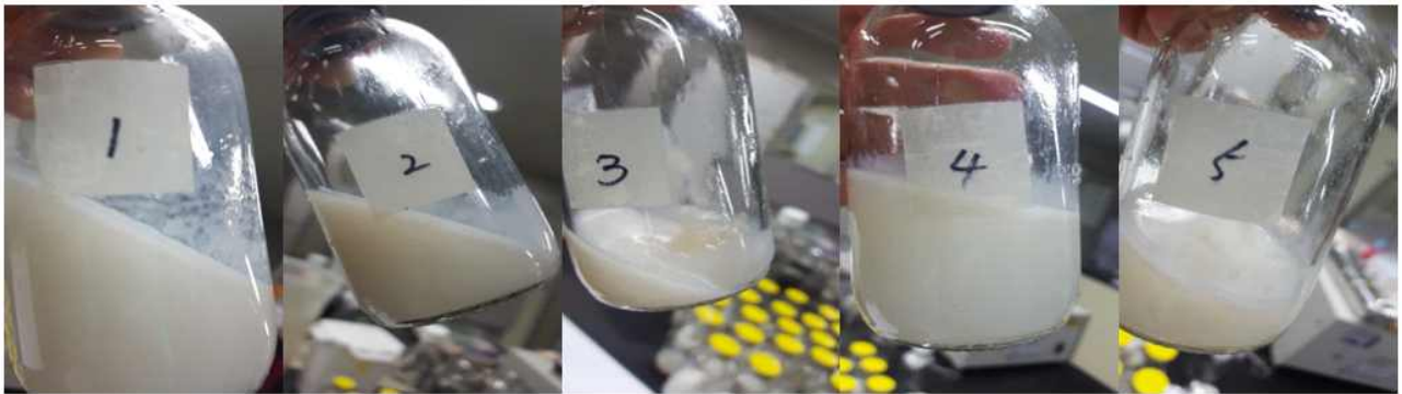
S30, 3%(0.01%, C971P), PH6.17 S30, 5%(0.01%, C971P), PH6.23 S30, 10% (0.01%, C971P), PH5.96 S30, 3%(0.02%, C971P), PH5.79 S30, 5%(0.02%, C971P), PH5.98
