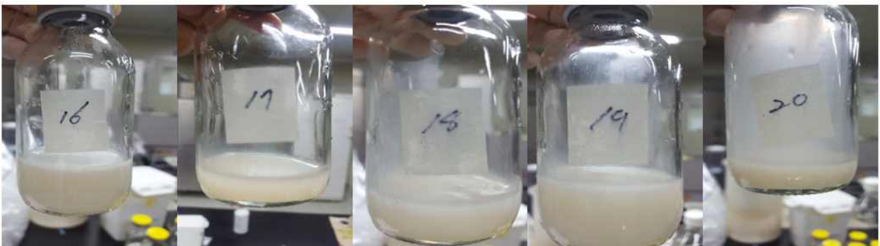
M20, 3%(0.01%, C971P), PH6.46 M20, 7%(0.02%, C971P), PH6.46 M20, 5%(0.02%, C971P), PH6.40 M20, 3%(0.02%, C971P), PH7.20 M20, 7%(0.01%, C940), PH6.54
