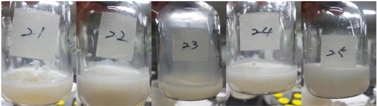
M20, 5%(0.01%, C940), PH6.51 M20, 3%(0.01%, C940), PH6.70 M20, 7%(0.02%, C940), PH6.40 M20, 5%(0.02%, C940), PH6.24 M20, 3%(0.02%, C940), PH6.16
