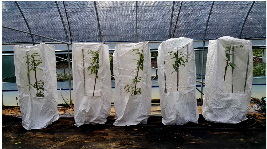
그림 26. Pipe frame cage (47.0 L × 47.0 W × 115.0 L cm) used in deterrent experiment in greenhouse.
