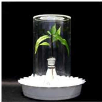
그림 25. Acrylic cylinder cage (25.50 H × 8.50 D cm) used in deterrent experiment in the laboratory.
