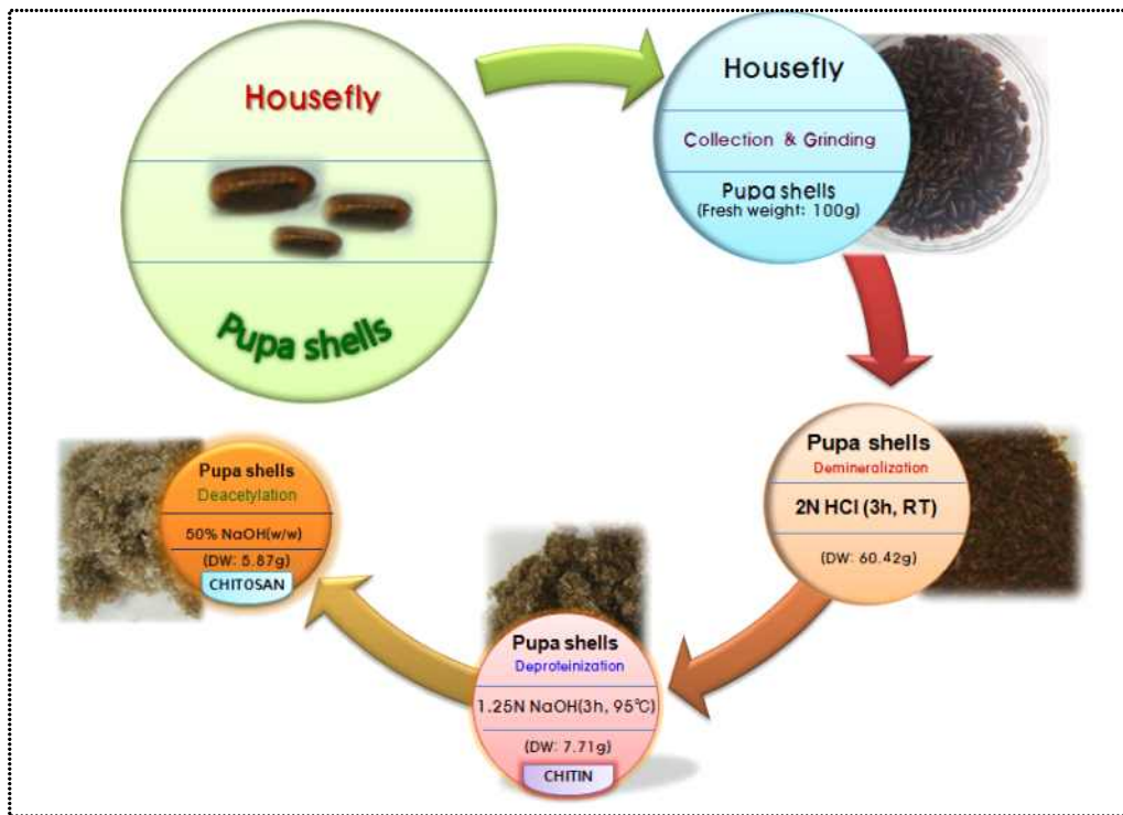
Fig. 1. Process for producing chitin and chitosan from housefly ( Musca domestica ) pupa shells.
