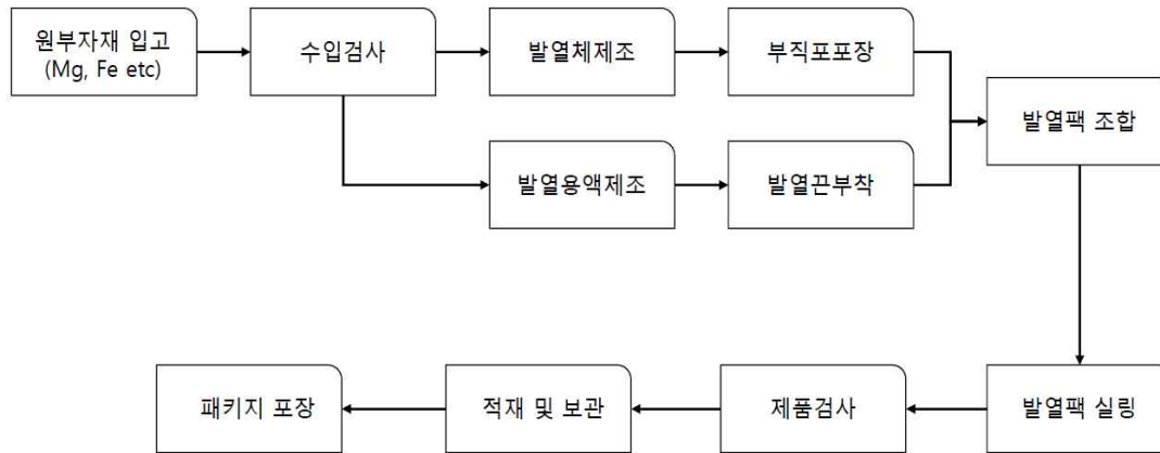
[그림23. (주)참맛발열팩생산공정Harvest charm food heat pack progress of production) ]
