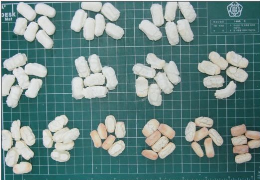
Fig. 11. Images of vacuum-puffed Yukwa from pellet moisture content of 20.17% at different heating time. (From left to right, top to bottom, the heating time is 1.33, 1.67, 2, 2.33, 2.67, 3, 3.33, 3.67, 4, 4.33, 4.67, 5, 5.33 min).
