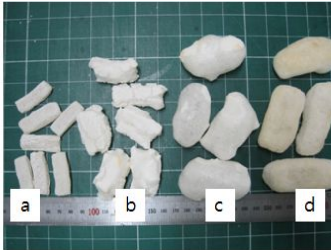
Fig. 9. Comparison with appearance of vacuum-puffed Yukwa under different release of pressure difference at 3 atm.
