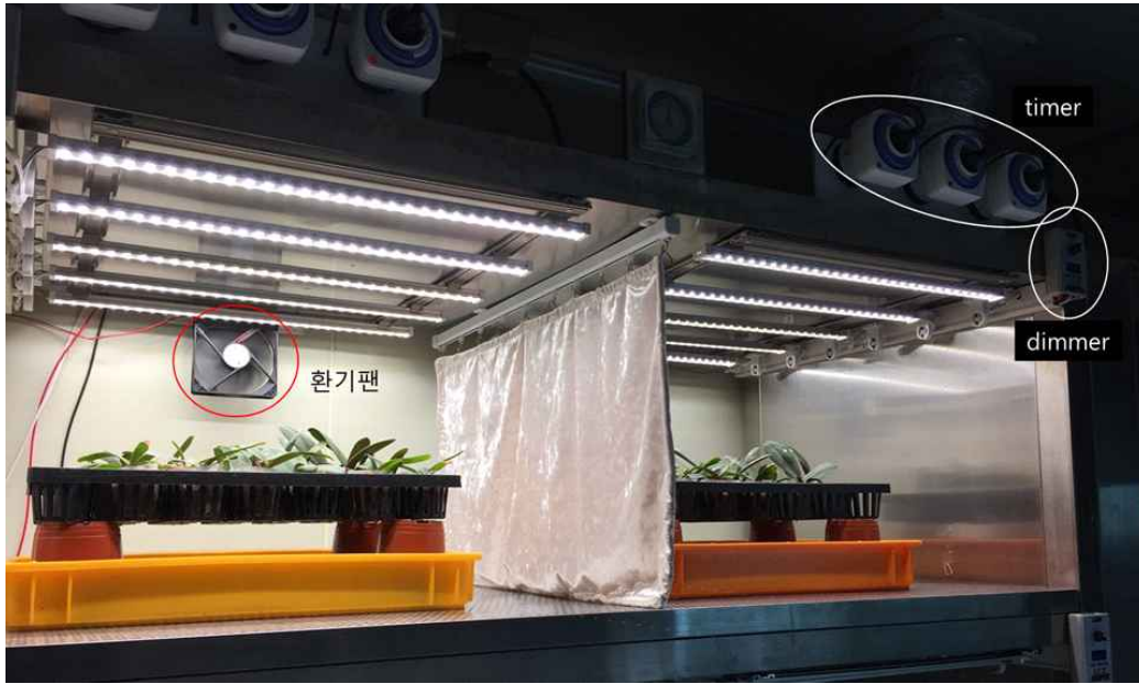
Fig. 3-2-2. Experimental beds for controlling light conditions in a closed plant production system.
