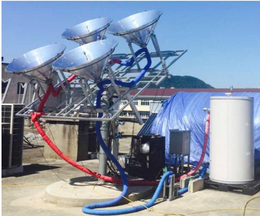
Figure 2-3 Experimental setup of conical solar concentrator system.
