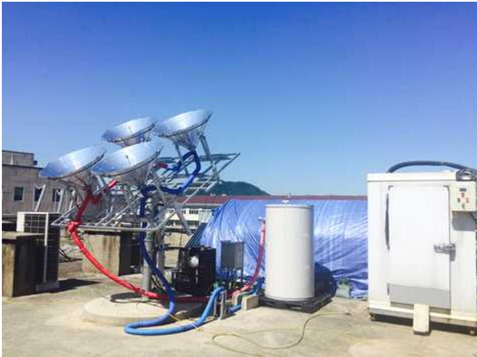
Figure 4-8. Experimental setup of dryer using conical solar concentrating system.
