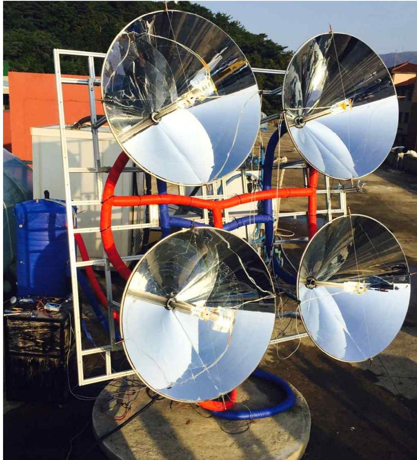
Figure 3-4. Experimental setup of multi module CPV/T conical system.
