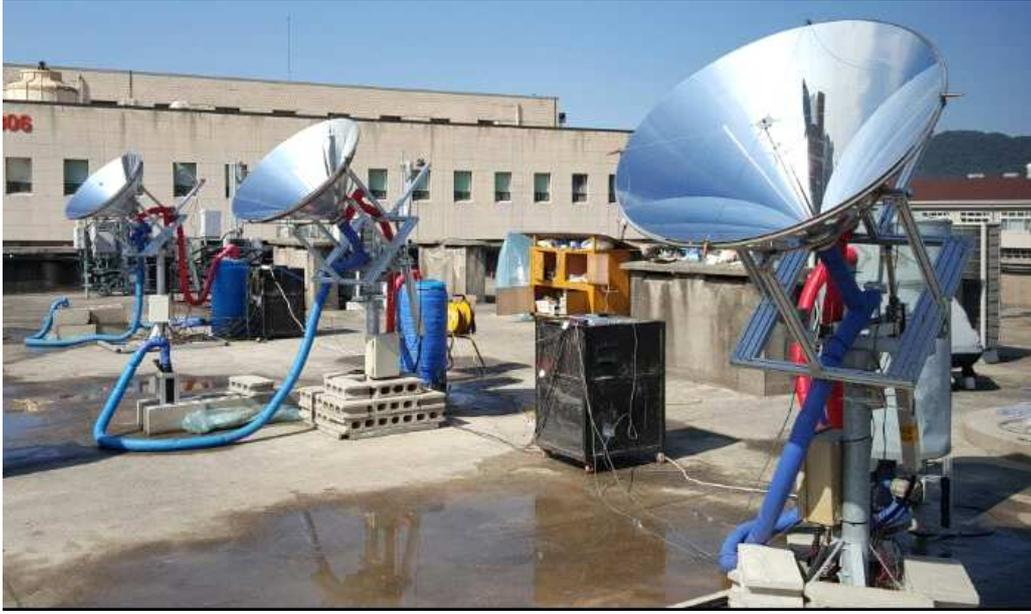
Figure 2-2. Experimental setup of conical concentrator system.
