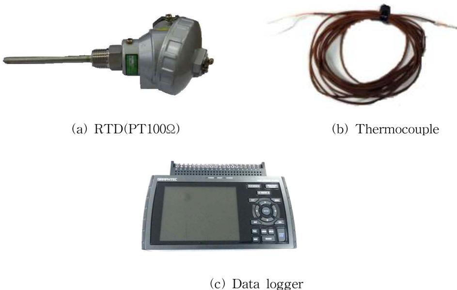
Figure 2-5. RTD, Thermocouple and Data logger.
