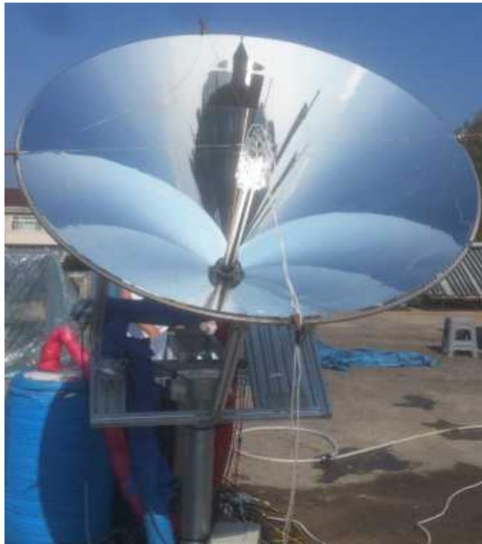
Figure 3-3. Experimental setup of single module CPV/T conical system.
