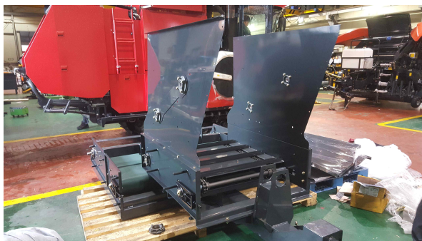
(c) Temporary storage tank (during assembly)
