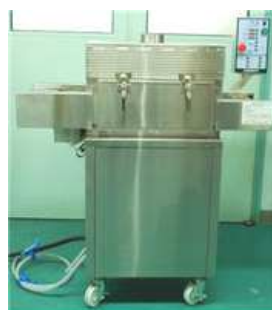
Fig. 8. 과열증기(Superheated steam) 설비
