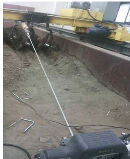
(b) Test rig hooked to winch
