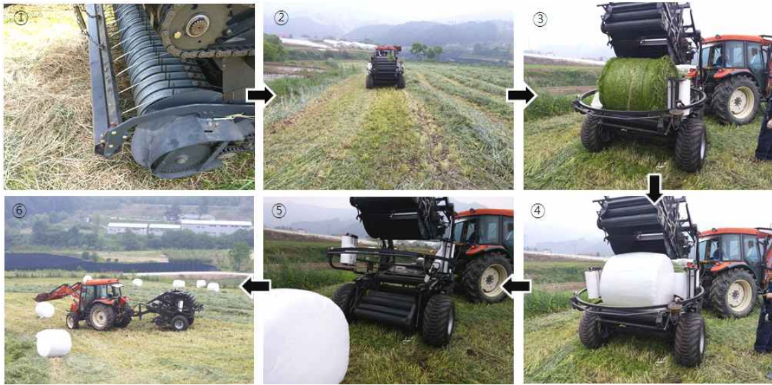
Figure 6. Performance test for tractor with an attachable integrated multi-purpose forage harvester (Rye-straw) (①Pick-up, ②Rolling, ③Netting, ④Wrapping, ⑤Discharging, ⑥Preparations and etc.)
