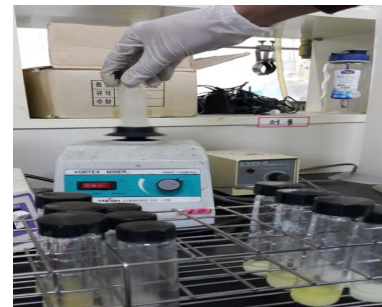
Fig. 1-13. The vortex process for measuring fatty acid composition
