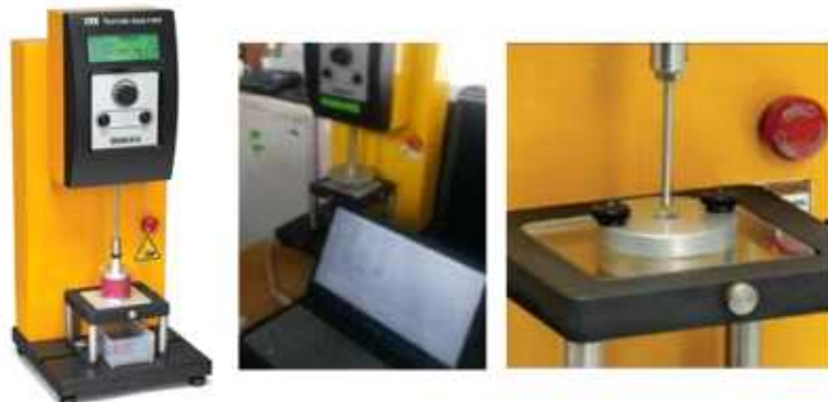
Fig. 4-21. Texture analyzer and TA-FSF probe.
