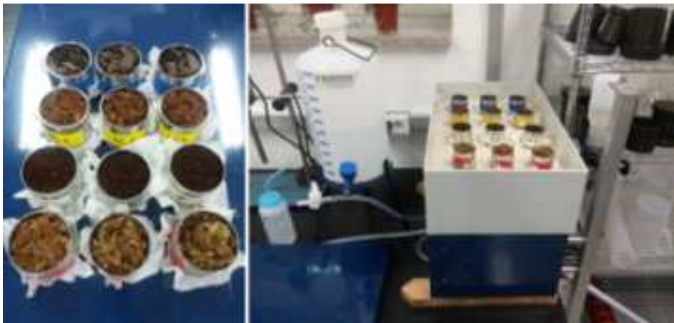
Fig. 1-34. Measuring moisture retention curve by using Sand box
