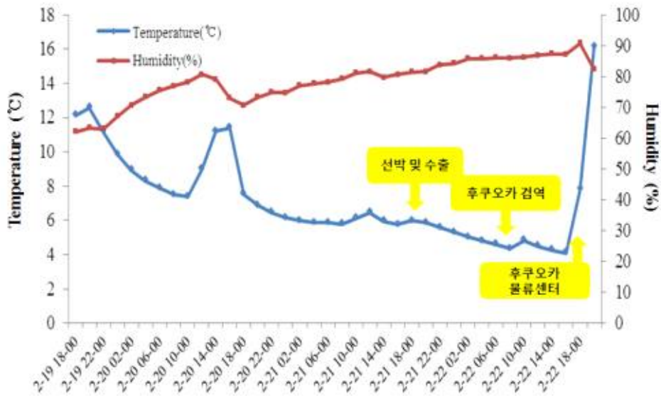
Fig. 2-40. Changes of temperature and humidity in the cut Cymbidium packaging box during shipping to Japan in Feb. 2017.
