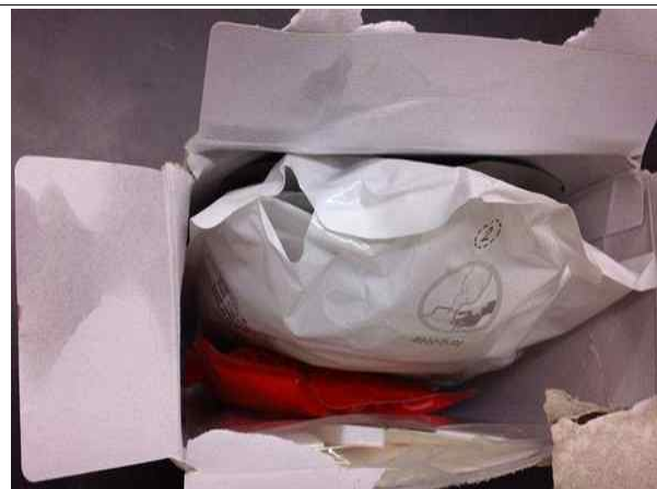
Seam failure at top of heater pack of the Type A product in Test 3.
