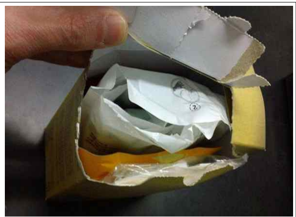
The seam failure at top of heater pack of the Type B product in Test 3.
