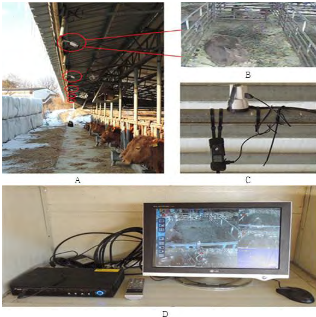
그림 60. Closed circuit camera, sound recorder and digital video recorder. A: closed circuit camera, B: an image of barn from closed circuit camera, C: real time recorder, D: digital video recorder monitoring system.
