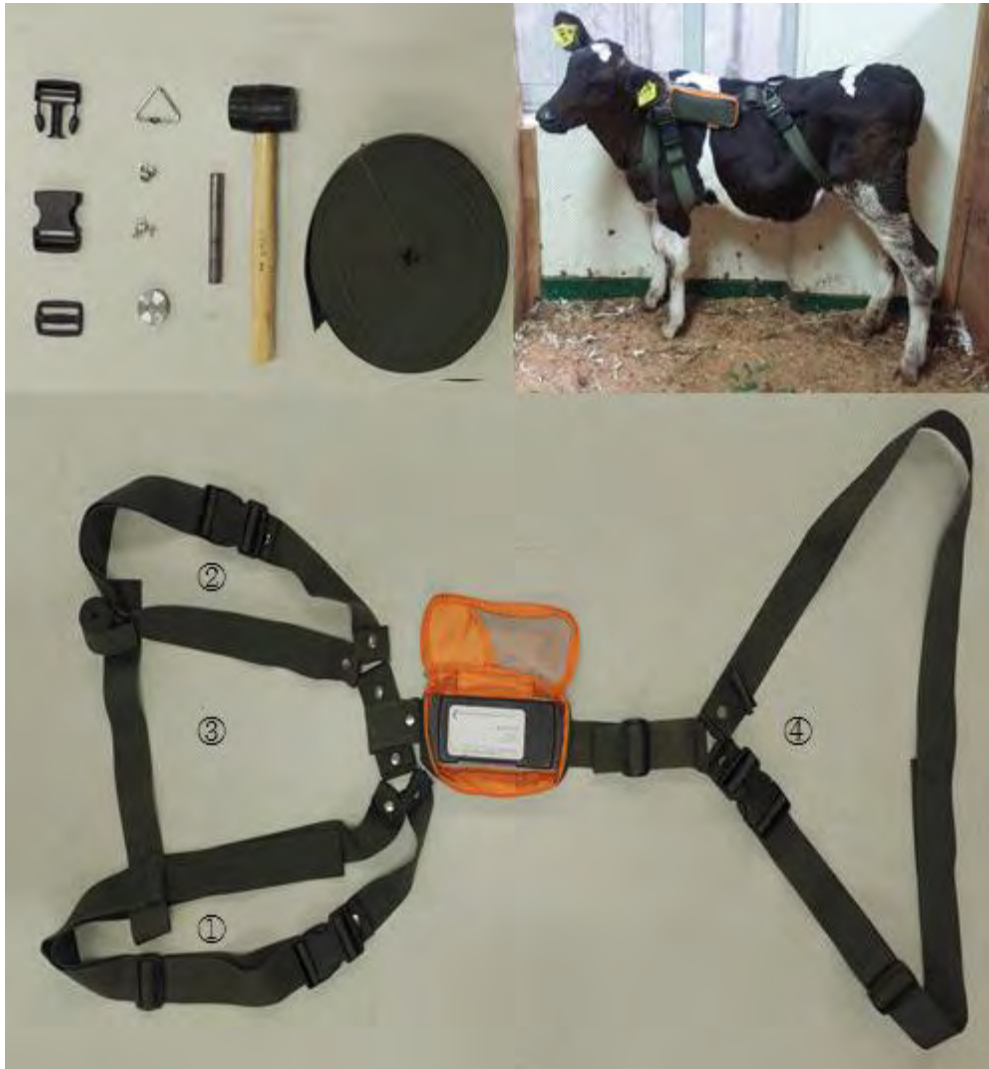
그림 38. Harness belt for body temperature measurement experiment of Holstein calf. Belt site ①: Left Leg, ②: Right Leg ③: Neck, ④: Abdomen
