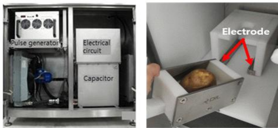
Fig 108. Inside view of 5 kW pulse generator (사진 좌) and batch chamber module with commercial 250 mL scale batch chamber (사진 우)
