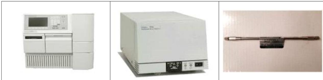
Fig.42. HPLC (Waters 2695), PDA(Photodiode array detector, Waters 996) 및 분석용 column
